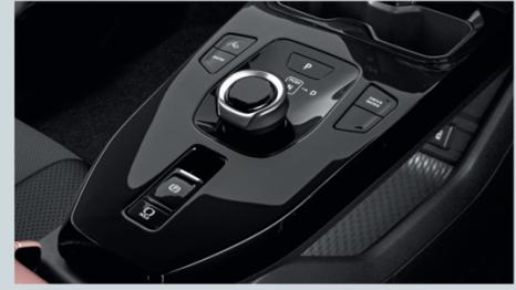
TWINDECK FLOATING CONSOLE WITH SHIFT BY WIRE
