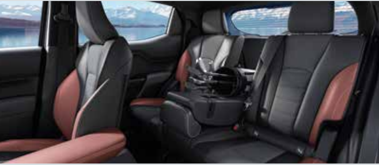
SEPARATELY FOLDING REAR SEAT BACKS (40:20:40 CONFIGURATION)
